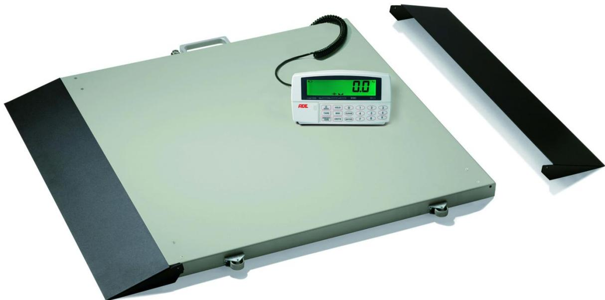
Low level platform scale with one ramp for convenient access with wheel chairs. A cable remote display shows the weight clearly and can be mounted to the wall. Two castors and one handle permit a quick transport. The pre tare function will allow you to deduct a memorized weight just by pressing one button. Such the net weight of a patient can be determined. A hold and tare function will help to get a quick and precise reading of the patient's weight. Powered by mains and rechargeable batteries.
